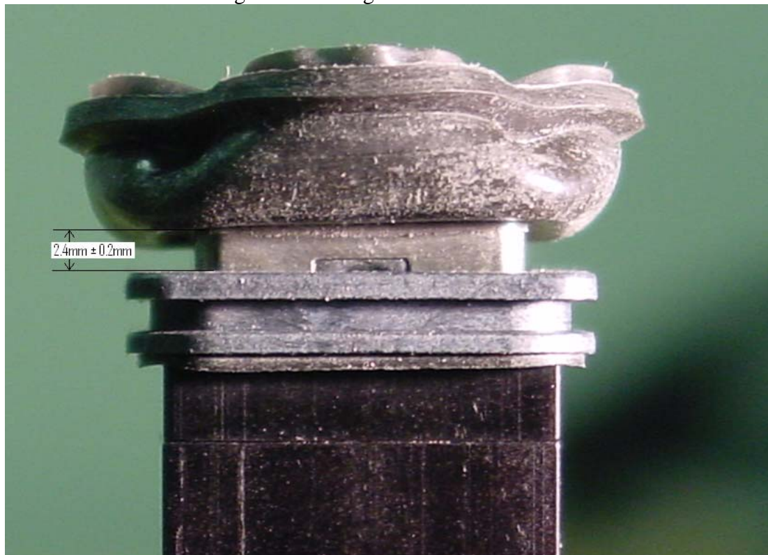
Figure 4 Pushbutton Depressed Alternate Position.
