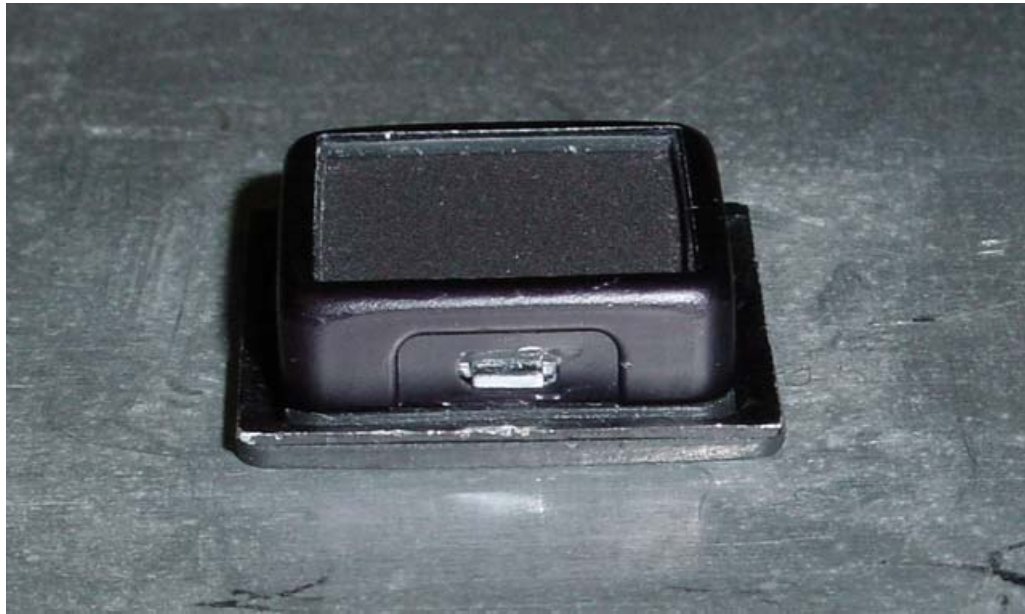
Figure 1. Unsealed and Splashproof Pushbutton.
