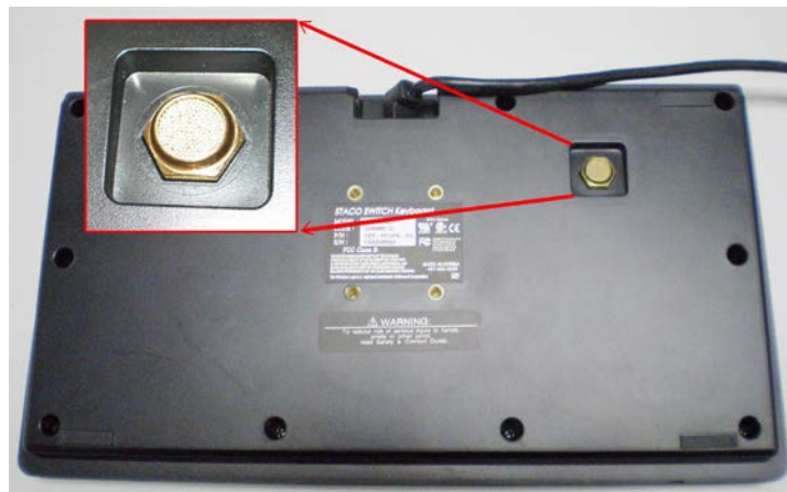
Fig. 4.2: Pressure relief vent in the back of the keyboard
