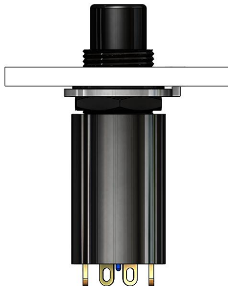
Figure 4: Switch Inserted in Panel
