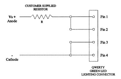
The recommended resistor value (R) and minimum resistor power rating  $(P_R)$  for a given power supply voltage source  $(V_S)$  are shown on the following table. Also shown are the minimum power supply power rating  $(P_S)$ .
